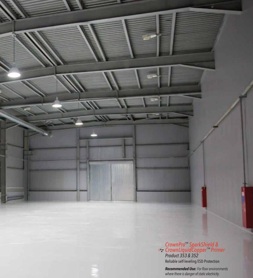
**System Description:** CrownLiquidCopper is applied as a self-leveling epoxy polymer concrete overlay and top coated with CrownPro SparkShield. The combination of the two products creates a high quality ESD system that complies with NFPA Static Dissipating Standards. The 2mm thick overlay also provides a tough wear surface that typically is applied at 3,000 ft<sup>2</sup>/hr.
